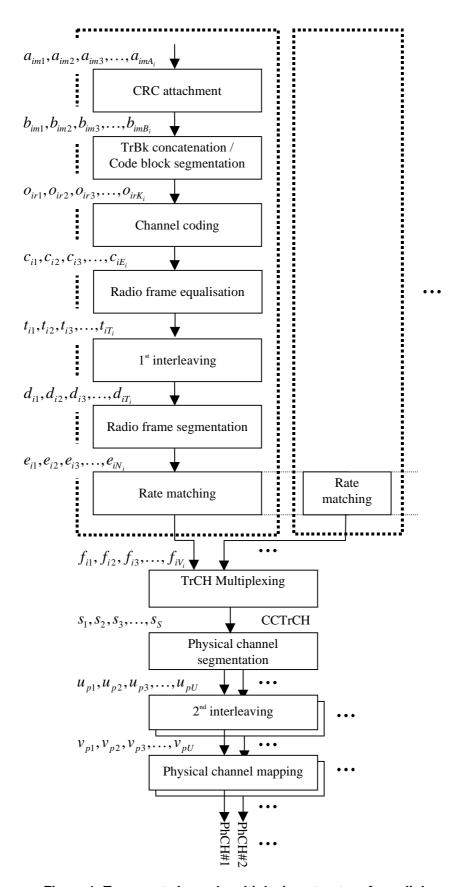
Figure 1: Transport channel multiplexing structure for uplink
